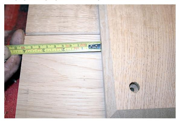
Place the bottom edge of the bottom ledge 7" from the door bottom.
