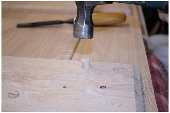
Using a sharp 1" wood chisel on its chiselled edge, remove the bulk of the plug excess.
