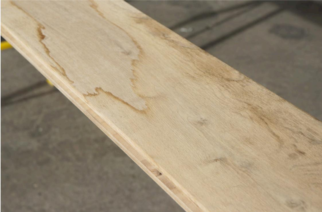
As mentioned before, the width of our engineered oak boards were 180mm. After heavy water damage, the width of the boards remained exactly the same.
